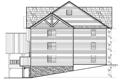
3 North Side Elevation A3 Scale: 3/32"=1'-0"
